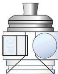
Glass reinforced nylon main body
